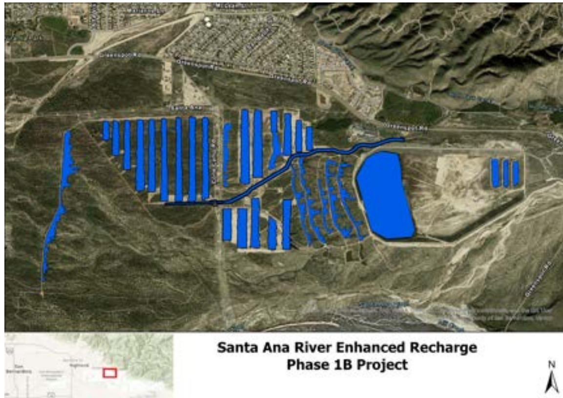
Figure 7-85 Groundwater recharge existing and proposed facilities below Seven Oaks Dam Source San Bernardino Valley
